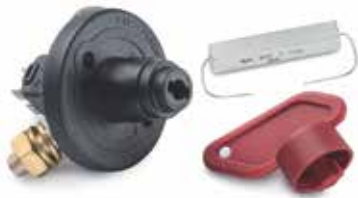
Battery master switch with rotating lever. Instant disconnection of all electric circuits. Provision for remote control Complies with FIA spec. Suitable for 6, 12 and 24V systems, rated at 100A continuous.
