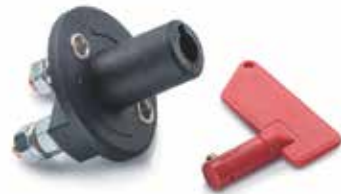
Bipolar master battery cutout switch with rotating lever. Instant disconnection of master electric circuit. Provision for remote control. Suitable for 6, 12 and 24V systems, rated at 100A continuous.
